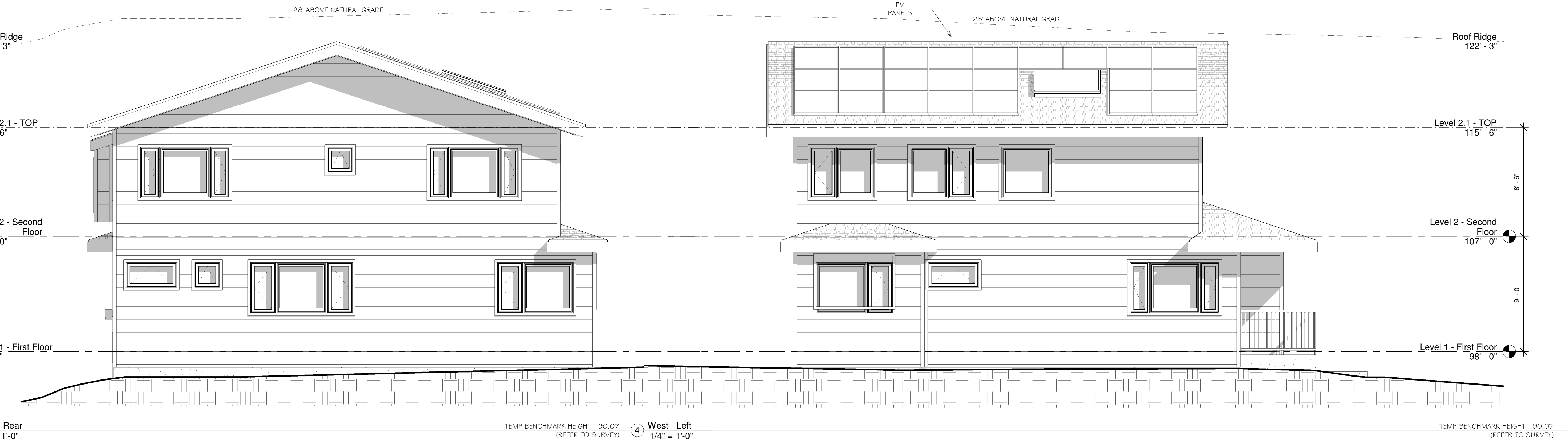
3 North - Rear 1/4" = 1'-0" TEMP BENCHMARK HEIGHT : 90.07 (REFER TO SURVEY) 4 West - Left 1/4" = 1'-0" TEMP BENCHMARK HEIGHT : 90.07 (REFER TO SURVEY)
