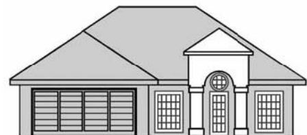
Entry is out of scale and has a commercial appearance.
