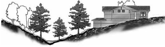
Structure is set back to avoid alteration of natural drainage feature
