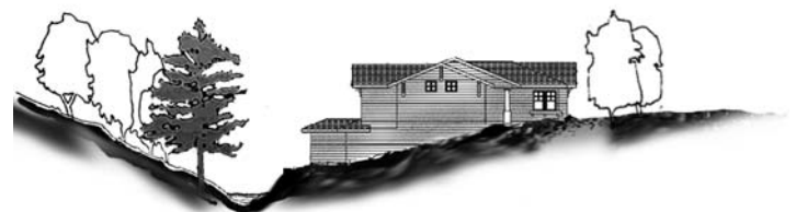
Structure is too close to natural drainage feature.
