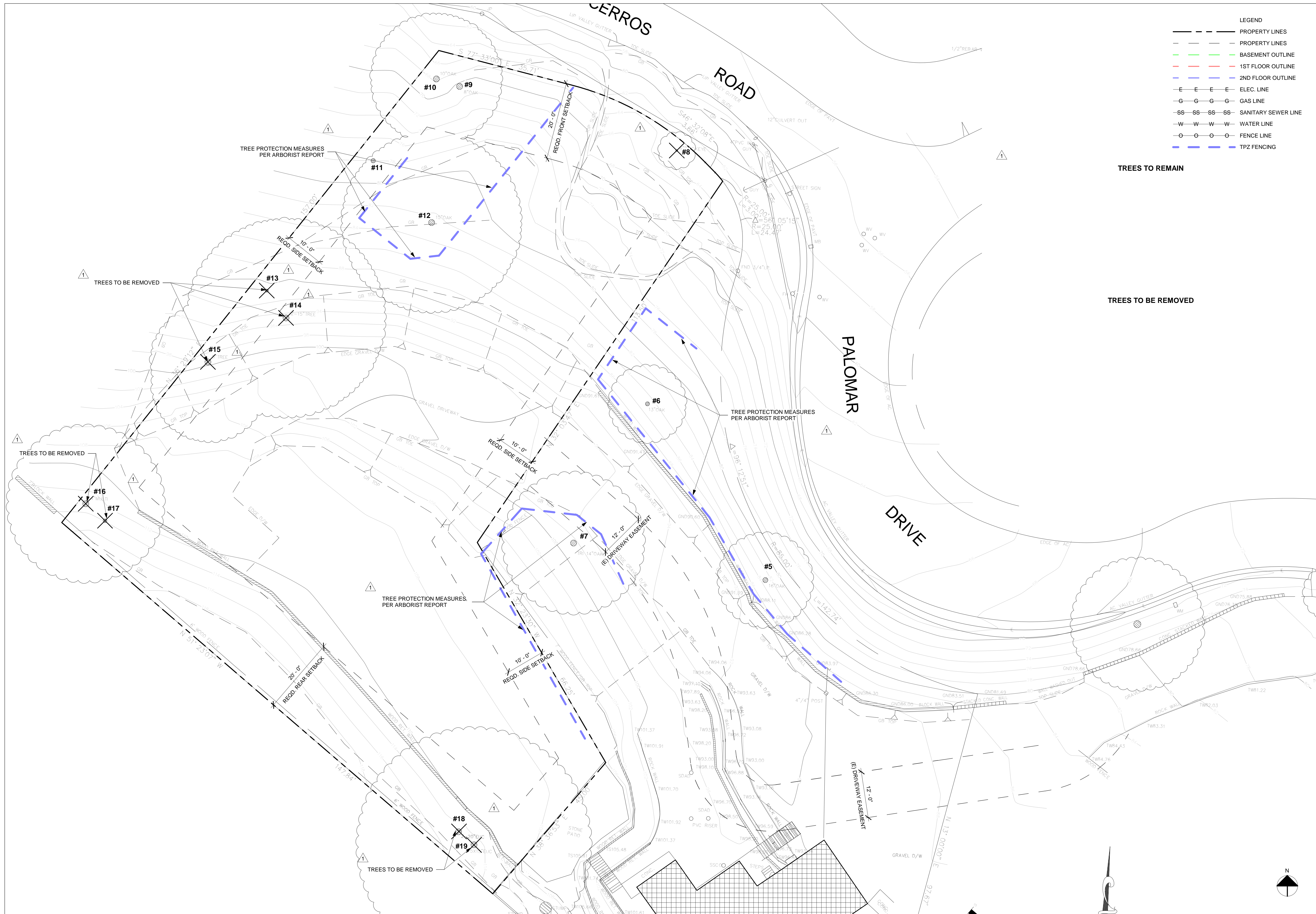
(E) SITE PLAN / TREE PROTECTION MEASURES
