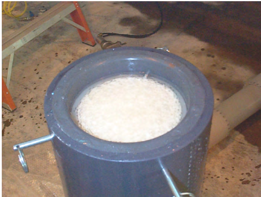
Fig 6-8 Testing the module for leaks
